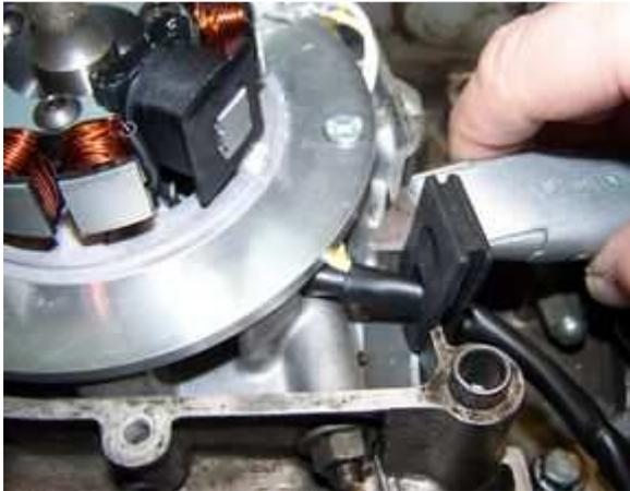
Push the rubber grommet with the cable in it into the opening .
