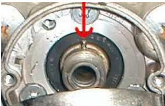
To find top dead center position (TDC) you may look at the camshaft, points end (after removing the points plate for points based systems). You will see the small pin in the index hole. At TDC it is straight down (or straight up), depending on cylinder.
