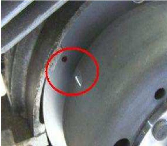
With the crank at TDC position of either of the 2 cylinders (no matter which), take the rotor carefully off again without changing crank position.
