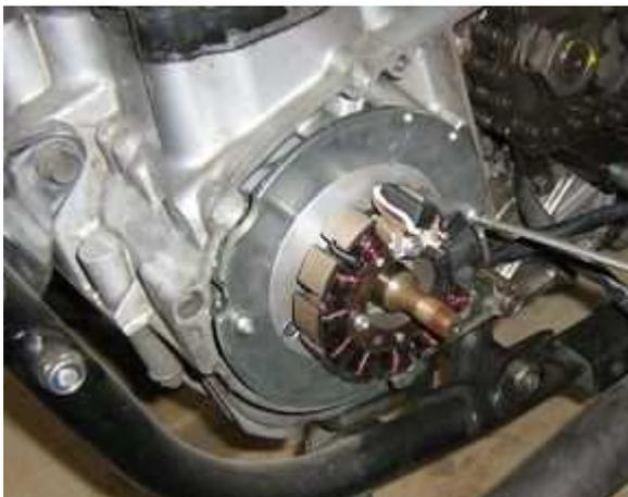
Place the new pre-assembled stator unit onto the engine block.
