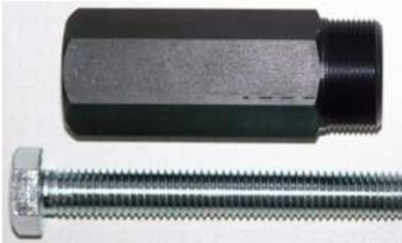
To disengage your new rotor again, you should use only the supplied special puller M27x1,25 (part-no.: 99 99 733 34).
