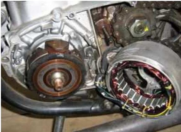
Disconnect the cables from your old alternator. Unscrew the old stator and take it off the engine. Pull the rotor off, you will need a puller screw for this.
