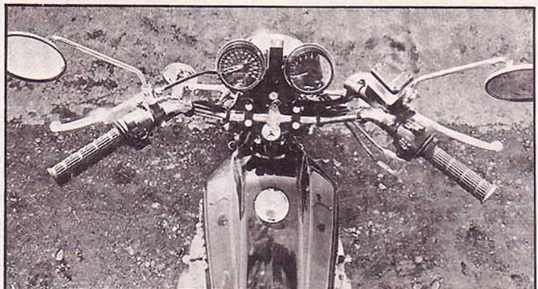
Above: Kawasaki's 'bars' are halfway to cowhorns and a reasonable compromise for the none too serious tourer/poser. Small filler cap is guaranteed to spill petrol. Low level fuel light is in tachometer.
