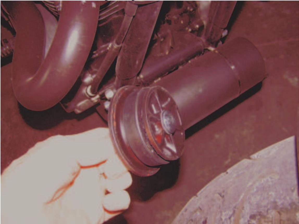
Use your imagination to mount the tube wherever it looks right. In these pics I added two stainless steel zip ties for looks but it also looks good as a plain 'tank'. I used two carriage bolts to attach it to the engine mount on this XS650.
