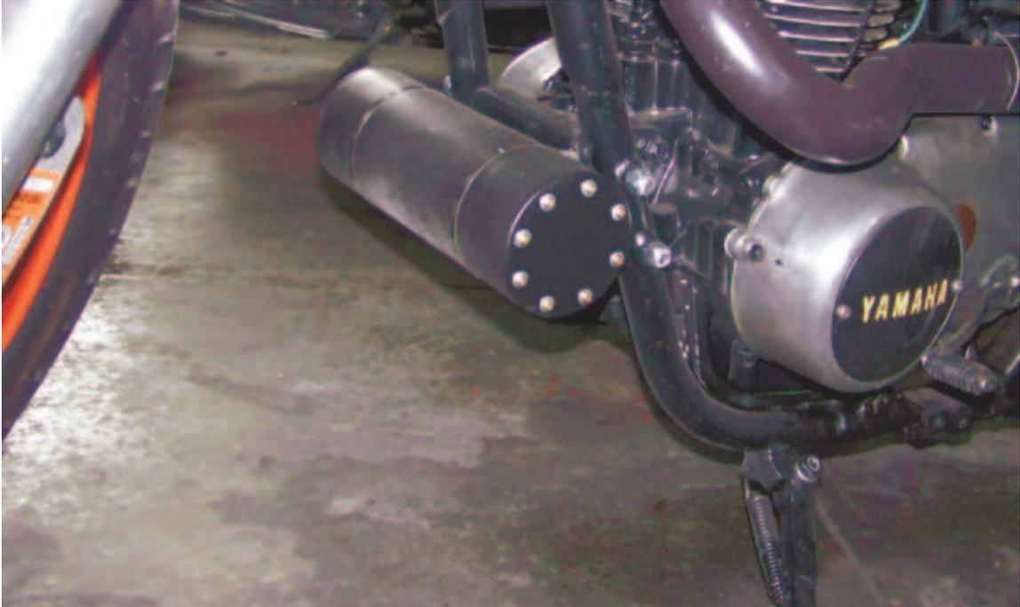
Made to resemble an oil tank it is constructed of rugged 3" PVC, permanently sealed on one end (with eight brass and steel 'rivets') and fully rubberized inside and out. The open end is sealed with a thermos bottle style expanding rubber cap and wing nut to keep water and dust out. This unit is 9" long although variations are available.
