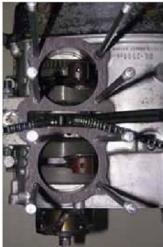
Figure 6-98: Secure chain, hang Cylinder
