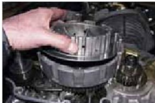
Figure 6-57: Inner part of the coupling used
