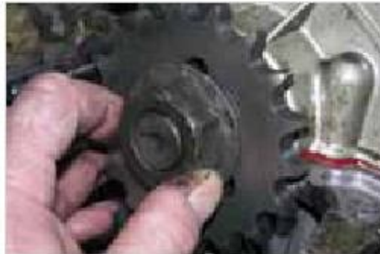
Figure 6-82: Pinion nut installed properly
