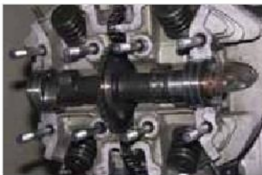
Figure 6-127: Replace camshaft
