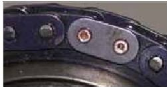
Figure 6-132: Chain lock - left rivet riveted already
