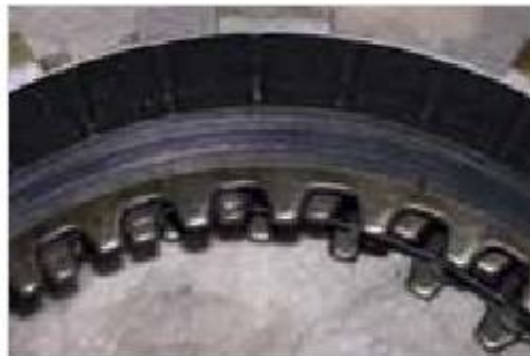
Figure 6-63: Clutch plates, rounded side out
