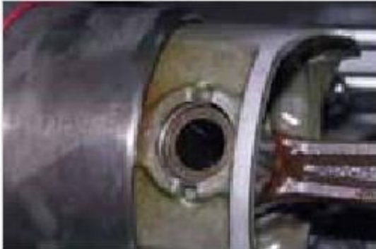
Figure 6-107: Piston pin and introduce secure (detail)
