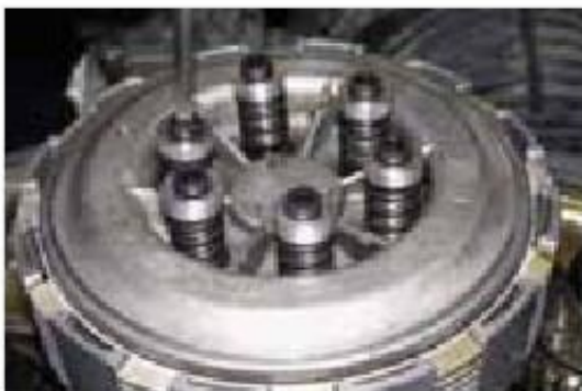
Figure 6-70: Compression springs installed
