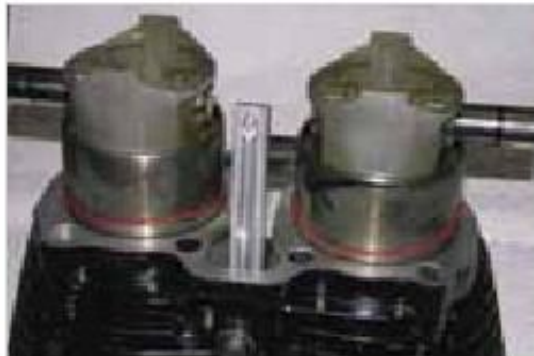
Figure 6-100: Sealing rings raise, Insert the piston pin from the outside
