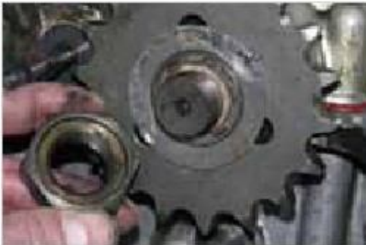
Figure 6-81: Pinion nut
