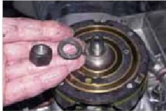
Figure 6-88: Rotor with spring washer and nut
