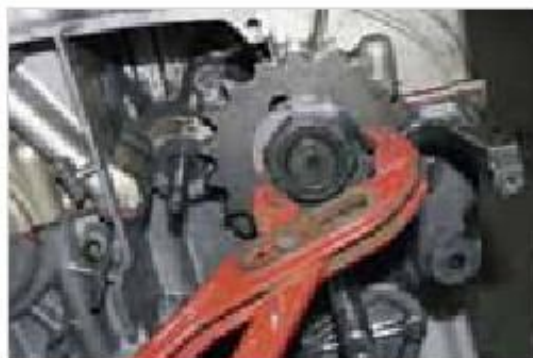
Figure 6-84: Locking plate bend
