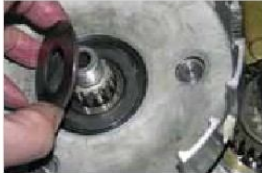
Figure 6-55: Insert bearings and thrust washer
