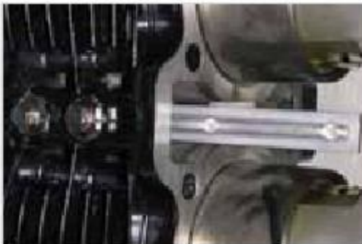
Figure 6-103: front timing chain tensioning rail mount
