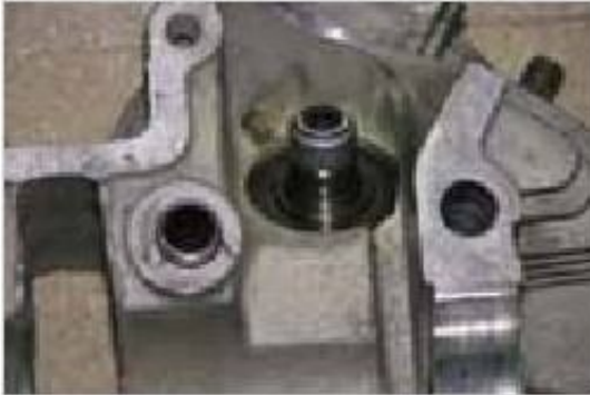
Figure 6-117: Put valve stem seal
