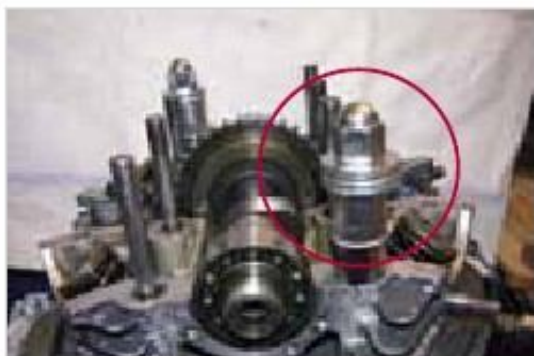
Figure 6-128: Cylinder block harness, the timing chain is usually too short to close it
