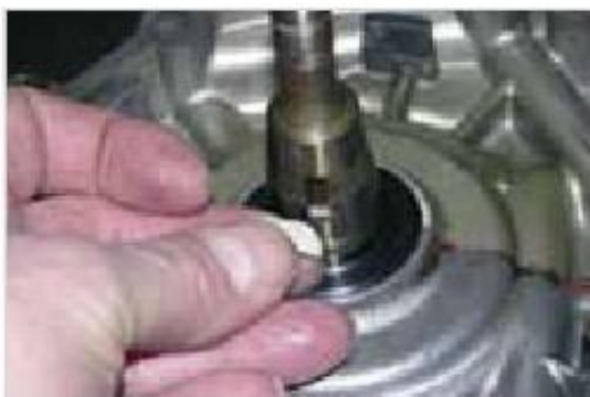
Figure 6-85: Rotor for disc spring into the groove in left crankshaft stump use
