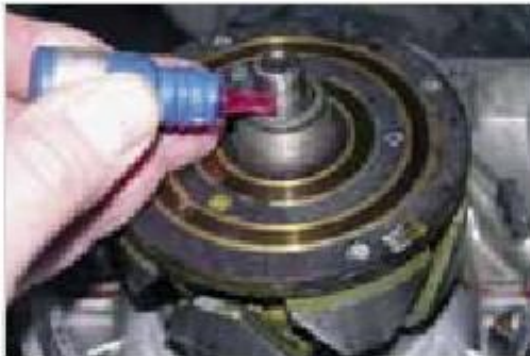
Figure 6-89: Apply liquid gasket
