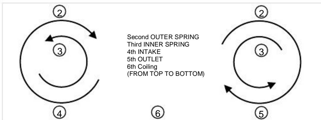
Figure 6-112: Orientation of the valve springs
