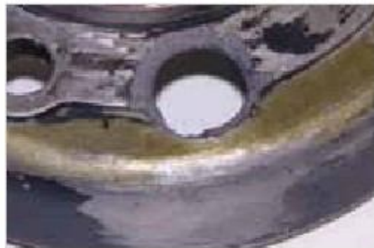
Figure 6-142: In Torn housing in the area of Reduction of the mounting screw due to an assembly error
