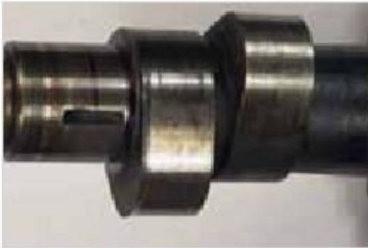
Figure 7-8: Worn cam in detail
