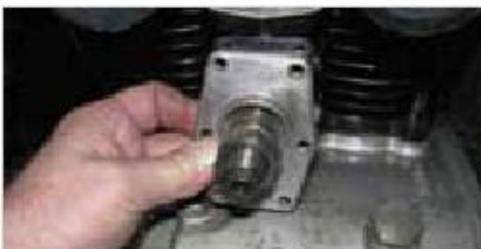
Figure 6-145: Timing chain tensioner mount
