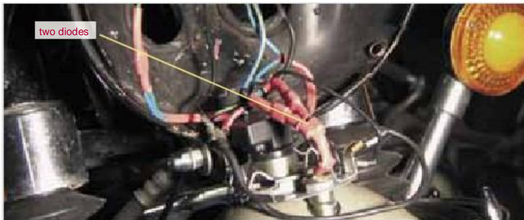
Figure 8-3: Cable to the parking lights with diodes
