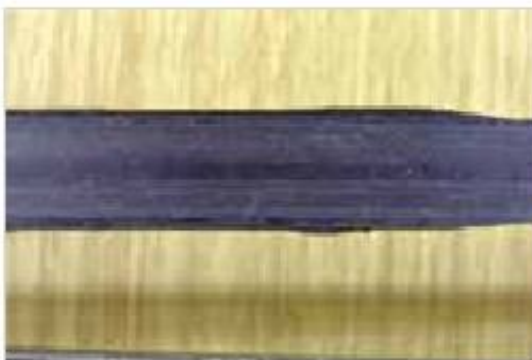
Figure 7-4: Wear of sliding surfaces in the image detail
