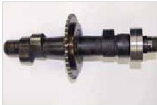
Figure 7-7: Camshaft with oil due to lack worn out cams
