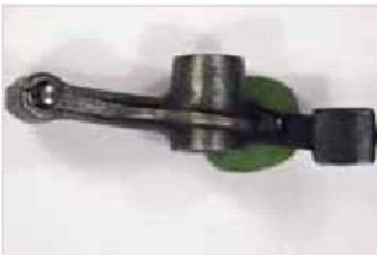
Figure 7-10: Associated sliding surface of a rocker arm
