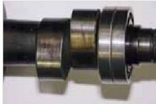
Figure 7-9: Worn cam in detail
