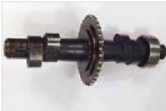
Figure 7-6: Camshaft with oil due to lack worn cam.
