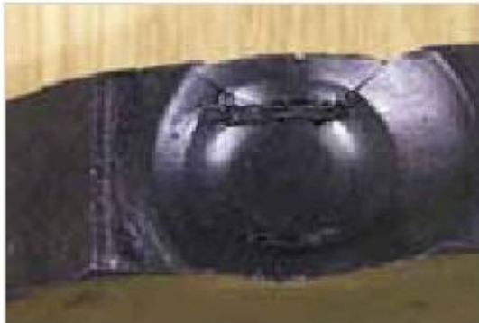
Figure 7-3: Spherical cap of the pressure bar the timing chain tensioner
