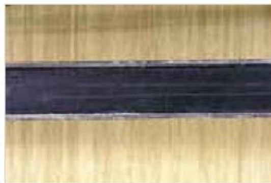
Figure 7-5: Wear of sliding surfaces in the image detail
