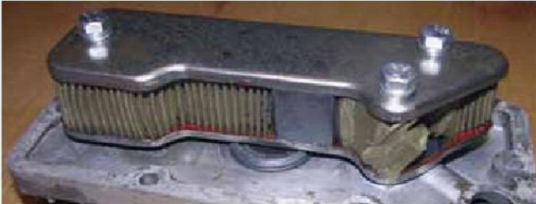
Figure 7-31: Oil filter with filter eingerissenem.
