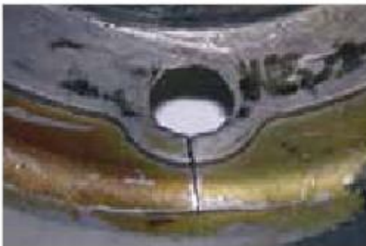
Figure 6-141: In Torn housing in the area of Reduction of the mounting screw due to an assembly error
