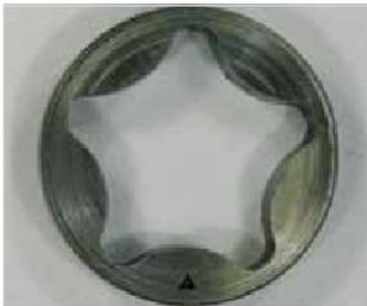
Figure 7-32: Outer rotor of oil pump
