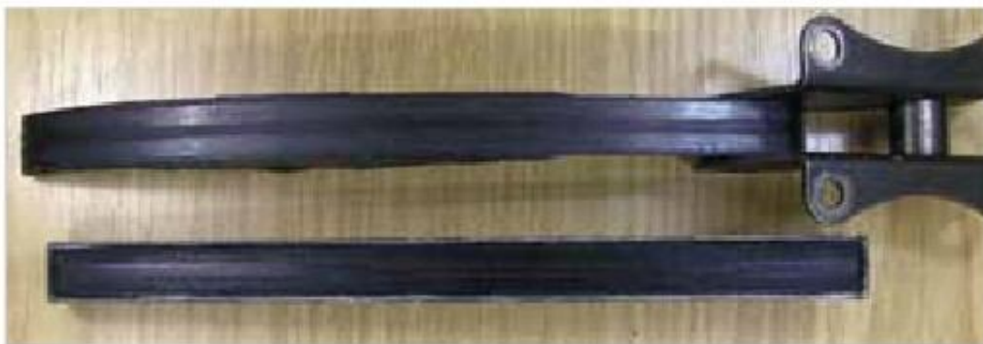
Figure 7-1: Sliding surfaces of the timing chain tensioning rail
