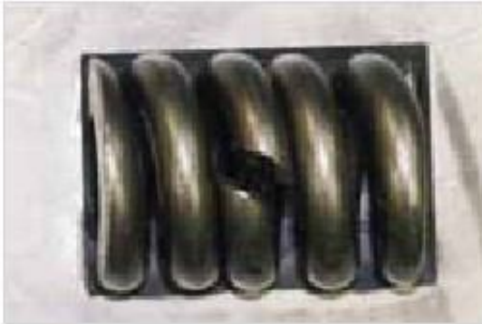
Figure 7-16: Broken damper spring
