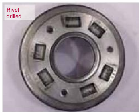
Figure 7-15: Back of the clutch basket with degraded shock absorber springs
