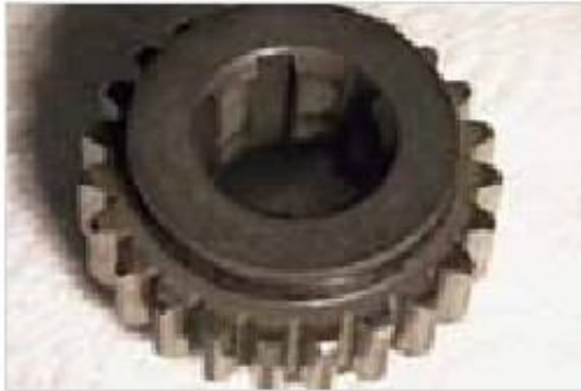
Figure 7-27: Gear of the fourth gear on the transmission output shaft
