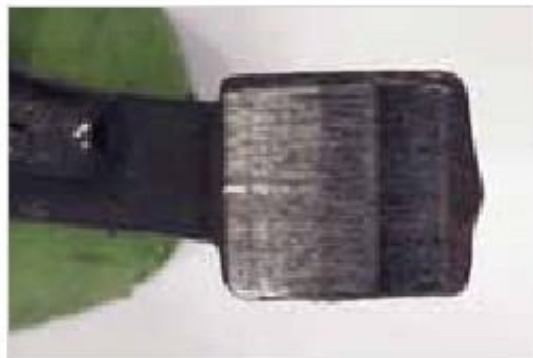
Figure 7-11: Associated sliding surface of a rocker arm
