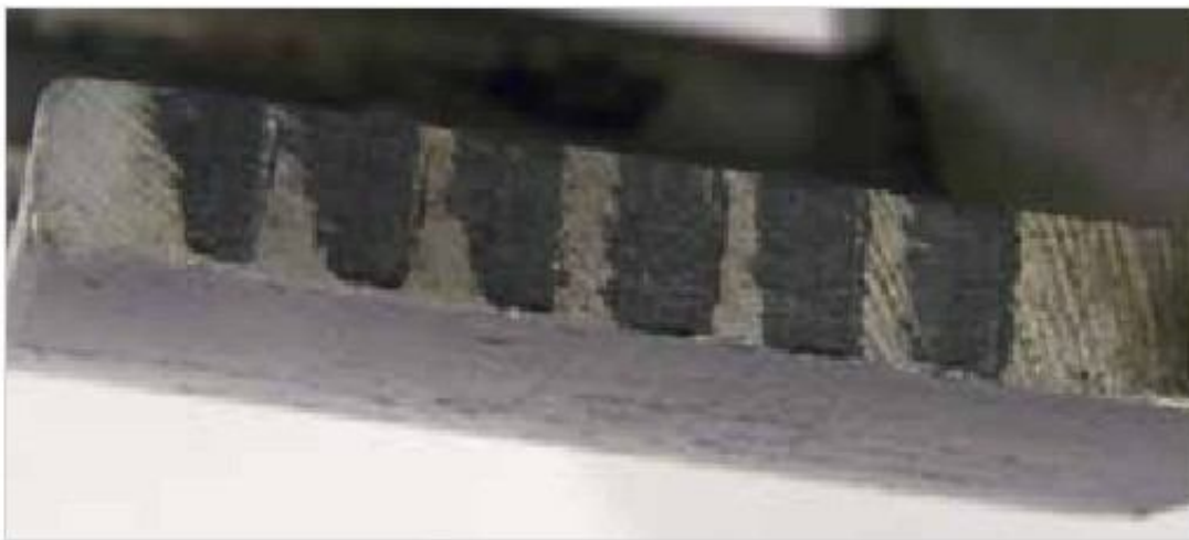
Figure 7-22: Impressions of the friction in the grooves of the outer clutch basket (enlarged detail)
