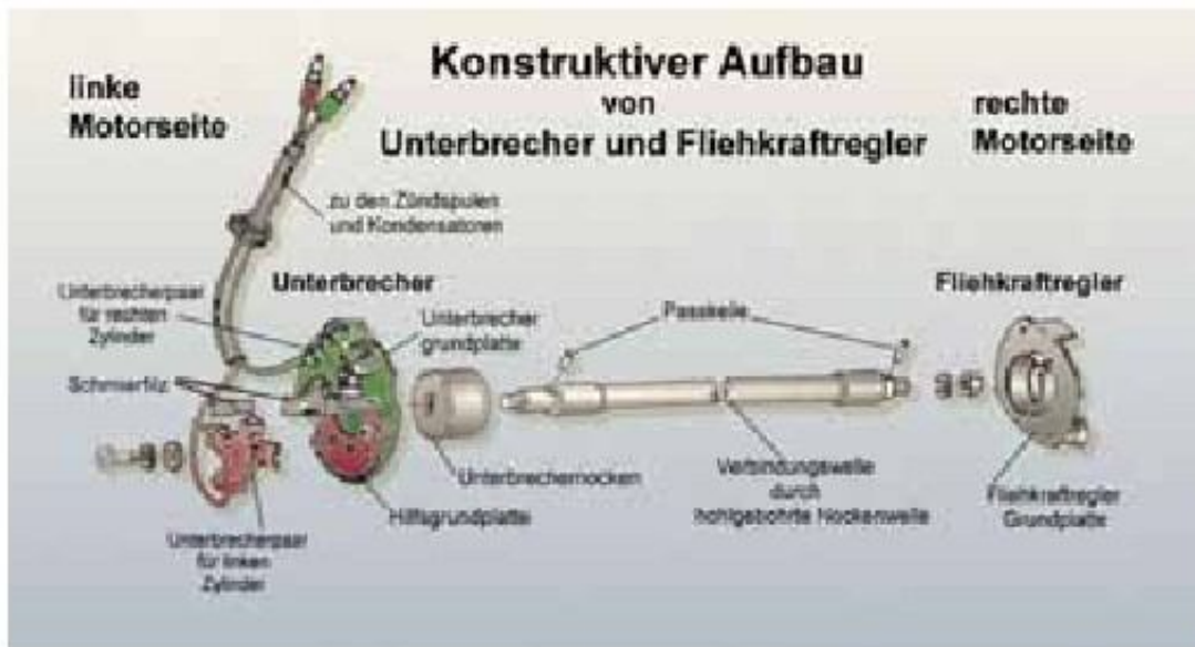
Figure 8-52: Construction of the interrupter and the centrifugal governor
