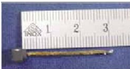
Figure 8-36: Carbon replica
