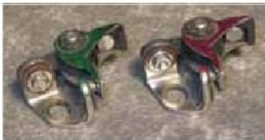
Figure 8-48: Contact pairs
