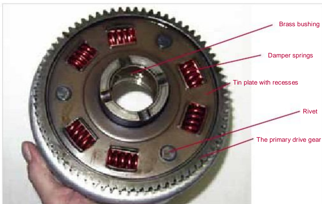
Figure 1-37: Outer clutch basket with 6 shock absorber springs
