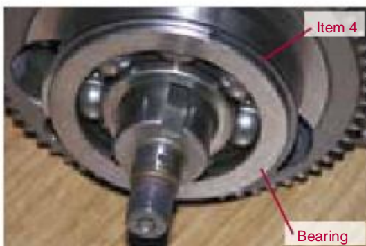
Figure 1-10: Output side of the crankshaft with right main bearing
