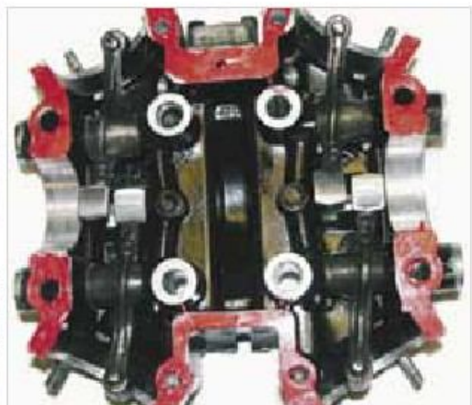
Figure 1-32: View in the upper part of the cylinder head
