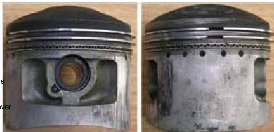
Figure 1-14: Piston with piston pin and snap ring inserted
