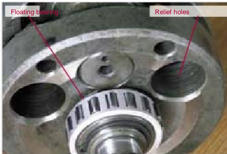
Figure 1-9: The generator side of the crankshaft
