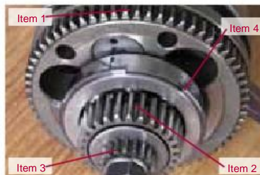
Figure 1-11: Output side of the crankshaft primary gear
