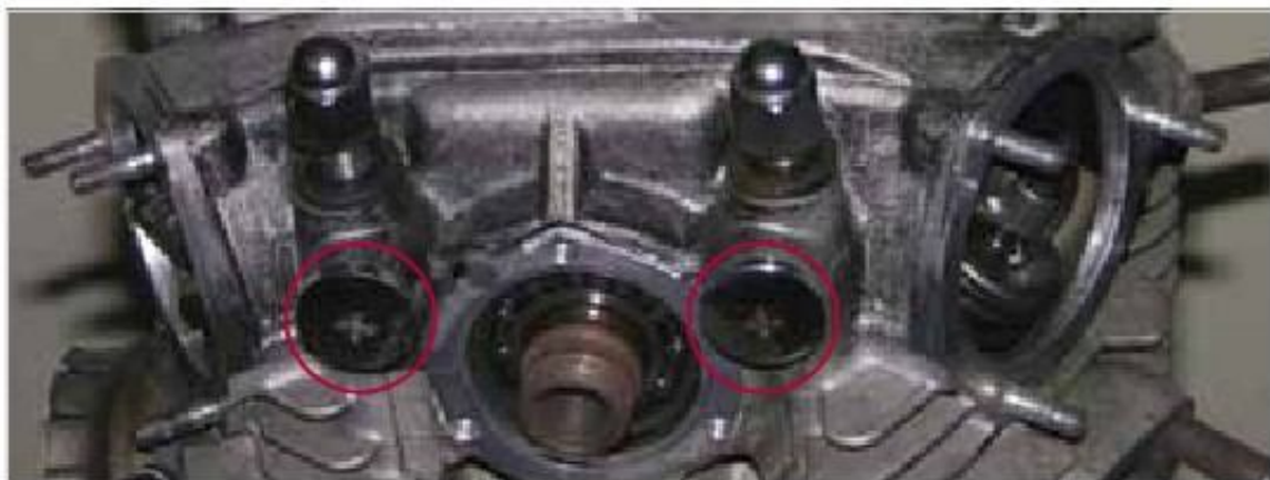
Figure 1-26: Storage of the rocker shaft
