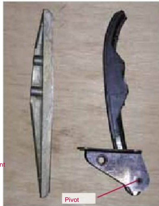
Figure 1-21: Timing chain tensoning rail
