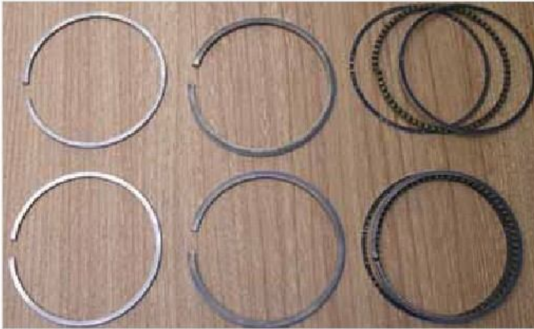
Figure 1-15: Piston Rings
