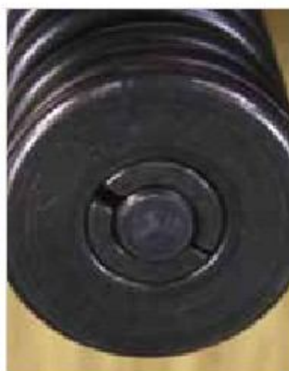
Figure 1-29: Valve plate valve wedges
