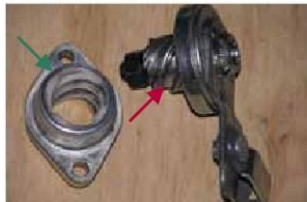
Figure 1-40: Disengaging the clutch in the dismantled State
