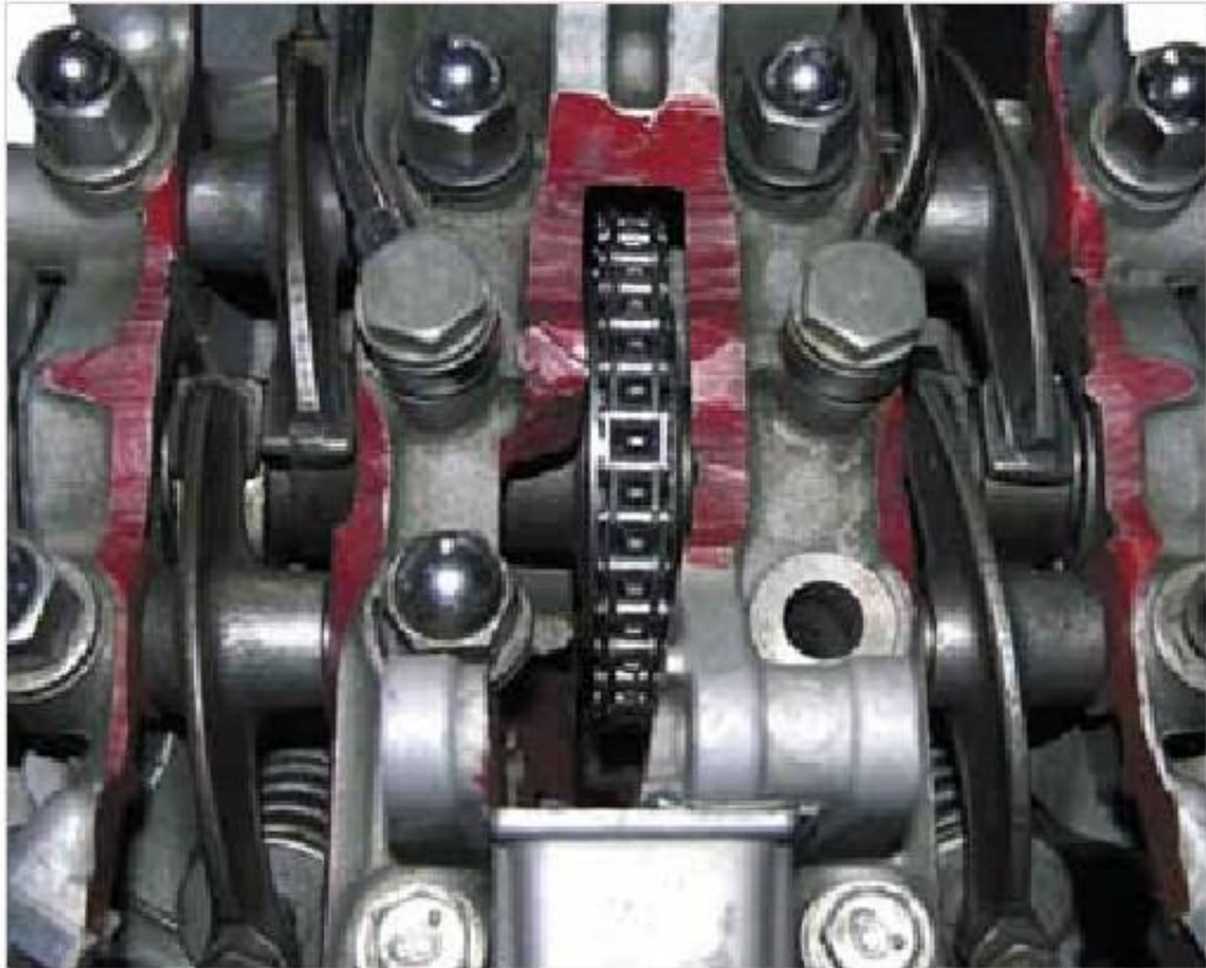
Figure 1-23: Camshaft and valve train valves
