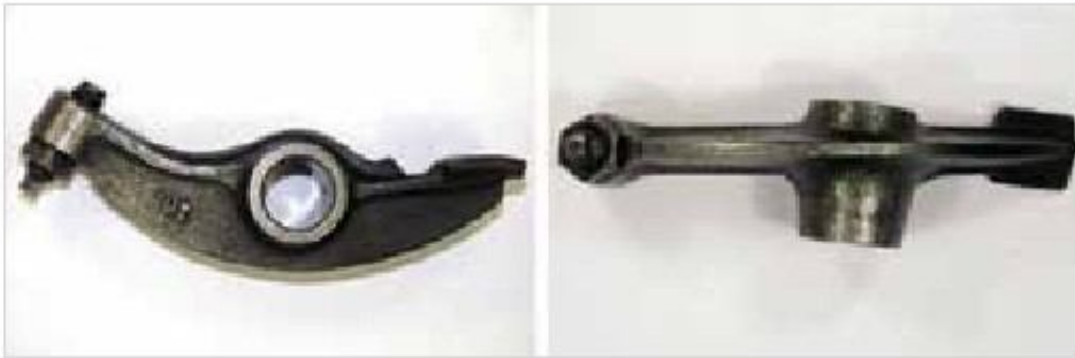
Figure 1-30: Rocker with Ventileinstellschraube
