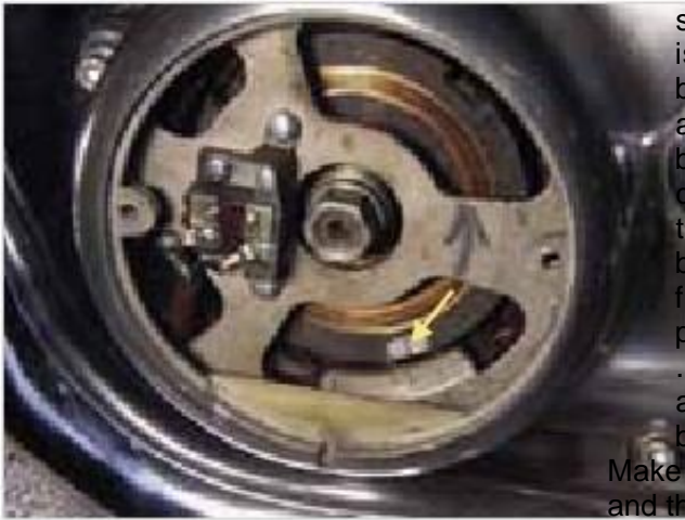
Figure 8-53: Timing mark
