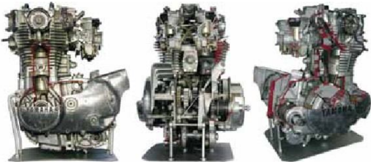
Figure 1-1: Cutaway model of the engine
