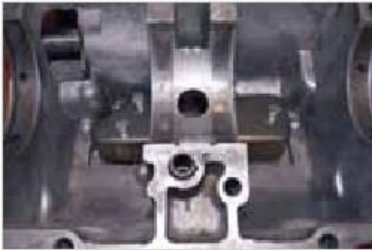
Figure 1-67: Installation of oil filter
