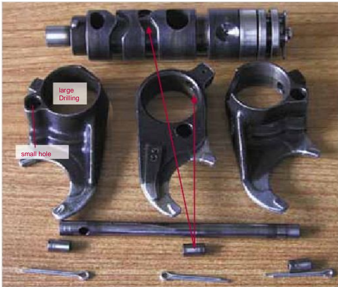
Figure 1-51: Shift drum
