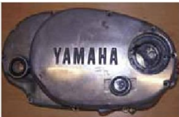
Figure 1-84: Right side engine cover with opening for the oil filter
