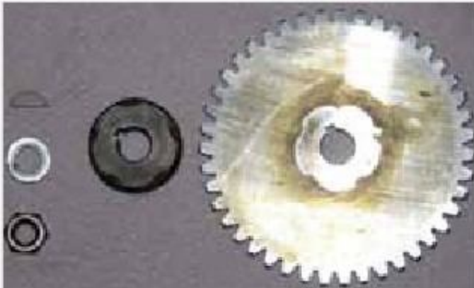
Figure 1-80: The oil pump drive gear and Screw drive the tachometer
