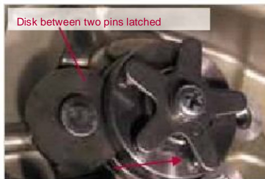
Figure 1-62: Gear is engaged
