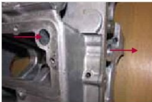
Figure 1-71: Oil passage between the oil filter base plate and right side cover
