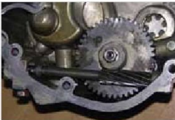
Figure 1-82: Tachometer drive
