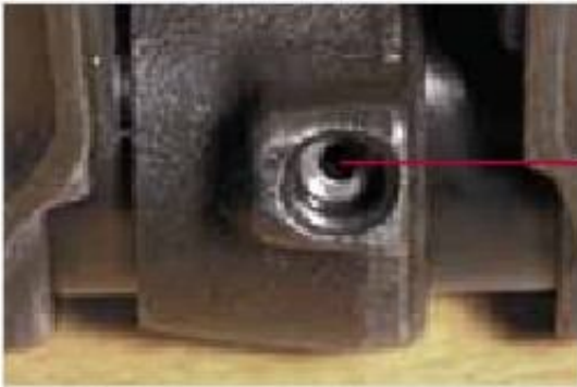
Figure 1-52: A shift fork guide pin
