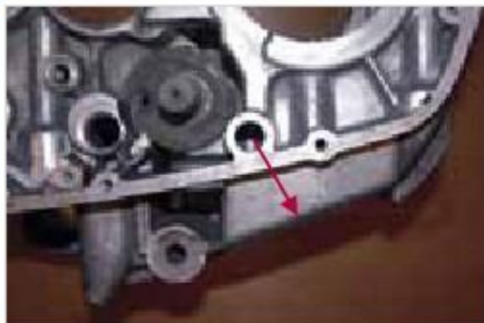
Figure 1-72: Outlet in lower engine housing section
