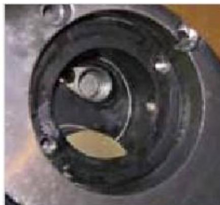
Figure 1-85: Opening for the oil filter in detail
