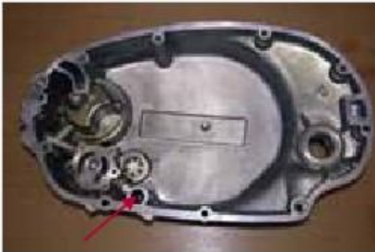
Figure 1-73: Inlet opening in the right side engine cover
