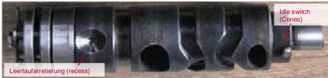
Figure 1-60: Cam switch with actuation for idle switch for deepening and bolts for Leerlaufarretierung
