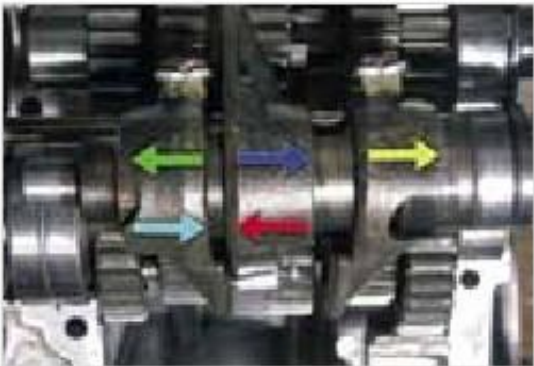
Figure 1-46: Assignment of the shift forks to the switching operations
