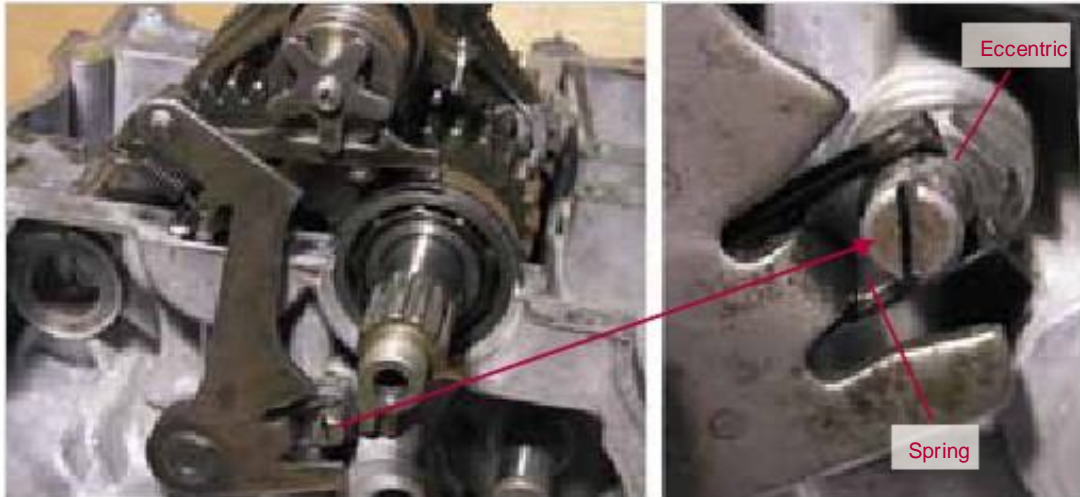
Figure 1-57: Setting the selector shaft
