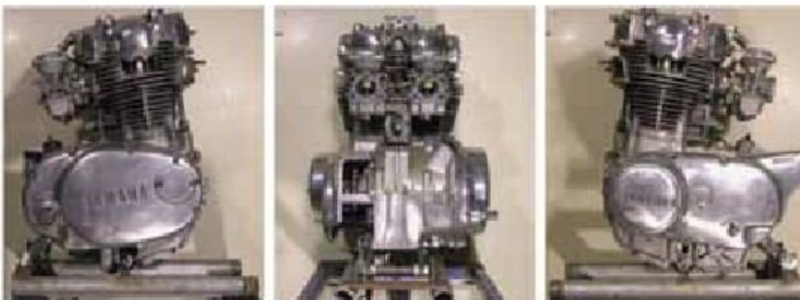
Figure 3-6: From pipes-built engine stand
