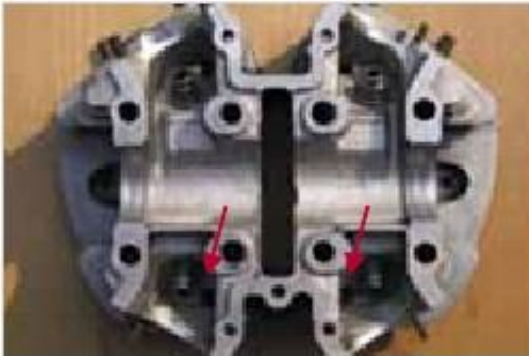
Figure 1-103: Oil drain holes in the cylinder head
