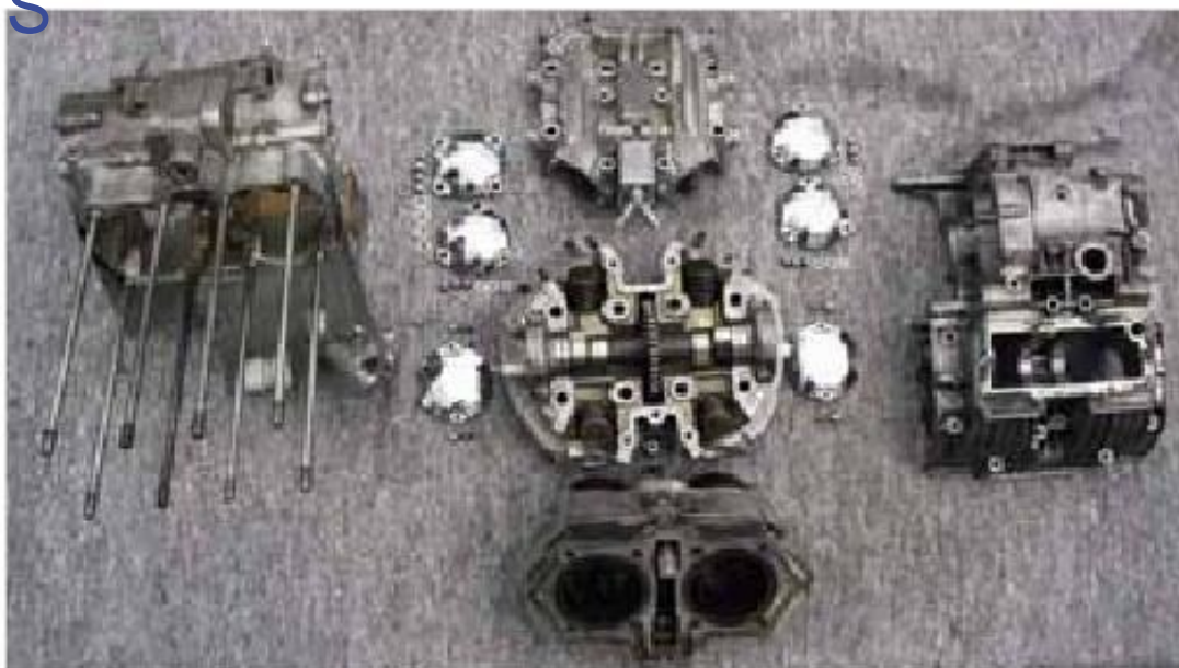
Figure 4-1: Housing halves, cylinder and cylinder head with camshaft
