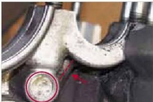
Figure 1-108: Oil pipeline through the Guide tube of the shift forks
