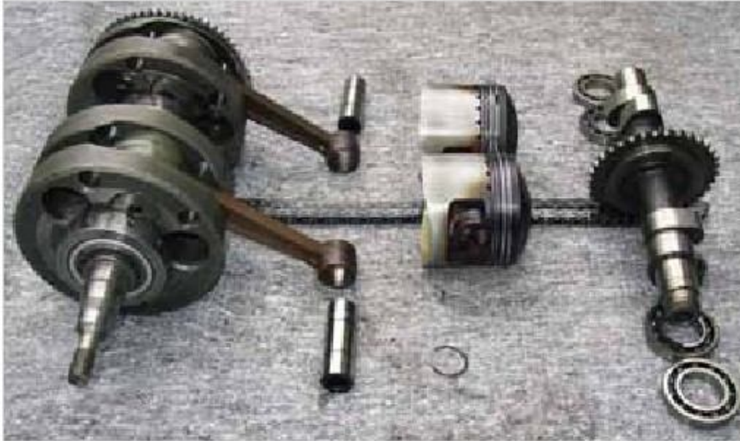
Figure 4-2: Crankshaft, pistons, timing chain and camshaft
