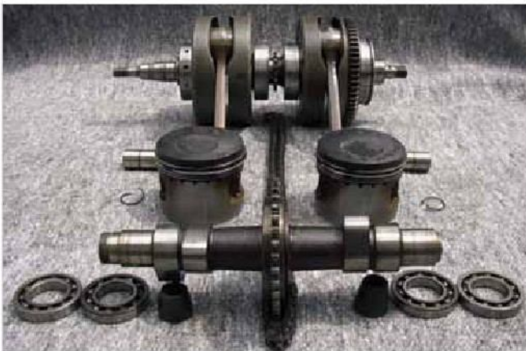
Figure 4-4: Crankshaft, pistons, timing chain and camshaft
