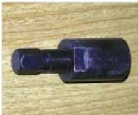
Figure 2-6: Puller for the generator rotor
