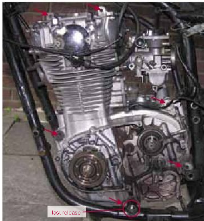
Figure 3-1: Attachment points of the engine under
