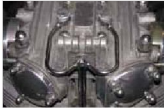
Figure 1-96: Connection oil riser / cylinder head
