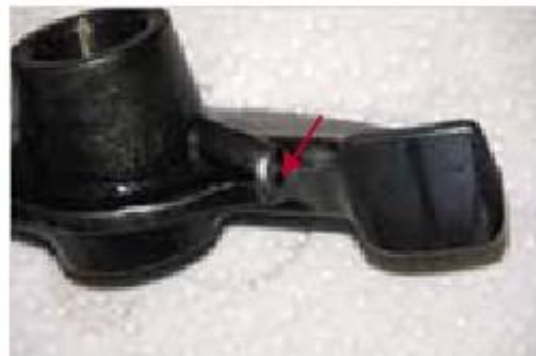
Figure 1-102: Oil outlet and Sliding surface of the rocker arm
