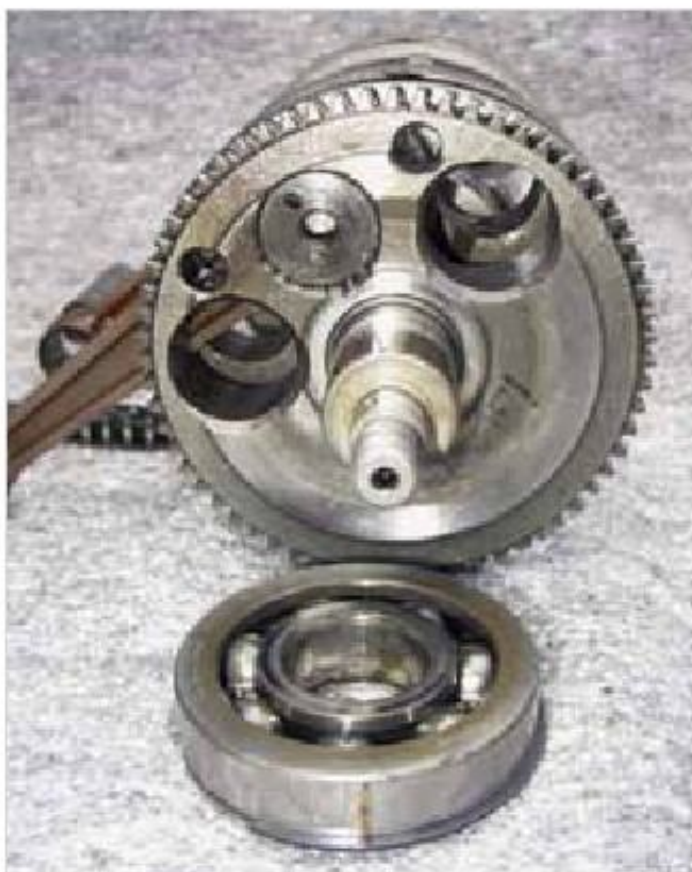
Figure 4-5: Bearing of the crankshaft
