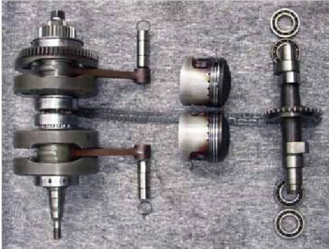
Figure 4-3: Crankshaft, pistons, timing chain and camshaft
