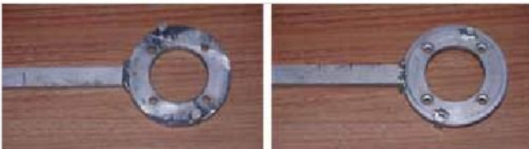
Figure 2-3: Tool for holding the chain sprocket
