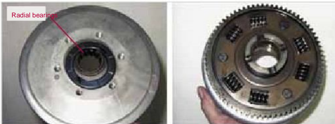
Figure 5-52: Front and back of the clutch basket with a radial bearing
