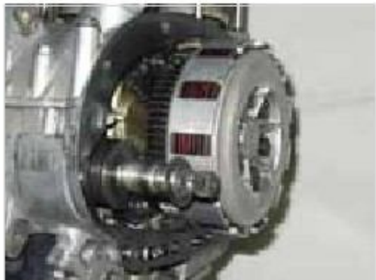
Figure 5-42: Pay attention to thrust washer, the kick starter shaft
