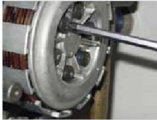
Figure 5-45: Clutch springs dismantle (Detail)
