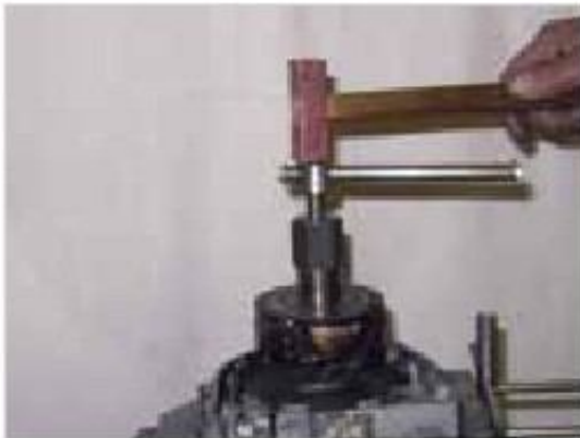
Figure 5-34: Remove rotor
