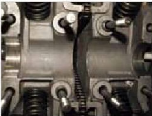
Figure 5-24: Timing chain secure, so that they do not slide off
