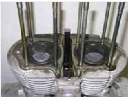
Figure 5-26: Cylinder with cylinder head removed
