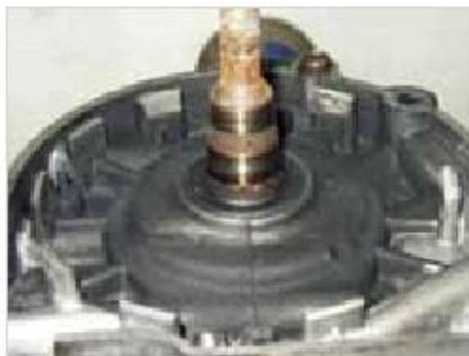
Figure 5-37: Rotor removed
