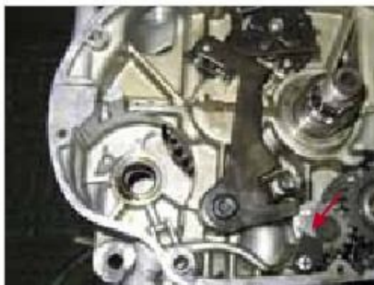
Figure 5-54: Kick starter mechanism pulled
