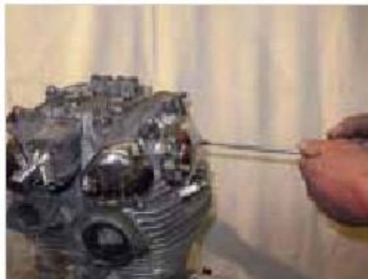
Figure 5-3: Removing the lid of the Contact set and of the governor
