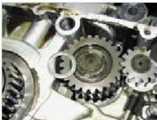
Figure 5-56: Remove gear
