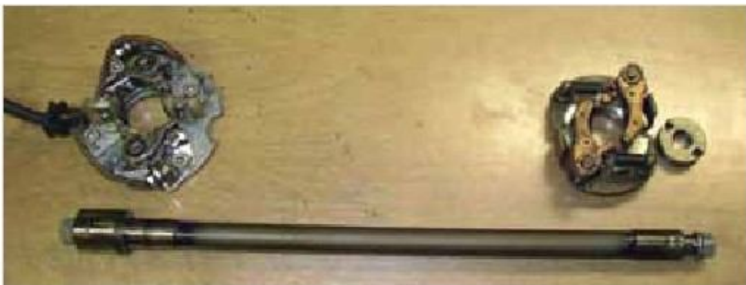
Figure 5-10: Parts of the interrupter and governor
