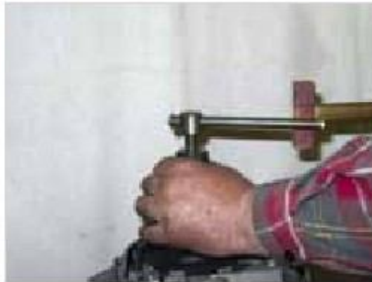
Figure 5-35: Remove rotor
