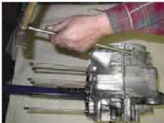
Figure 5-61: Housing halves separate
