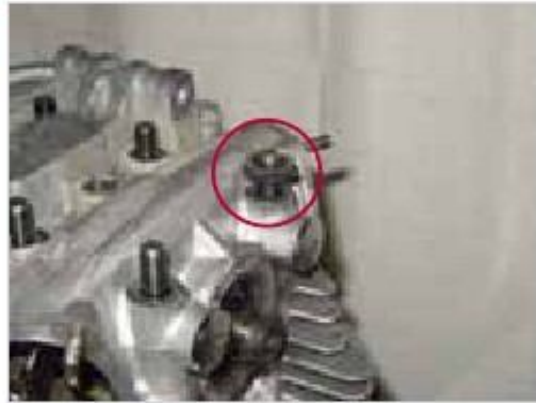
Figure 5-17: The outer plates are gummed
