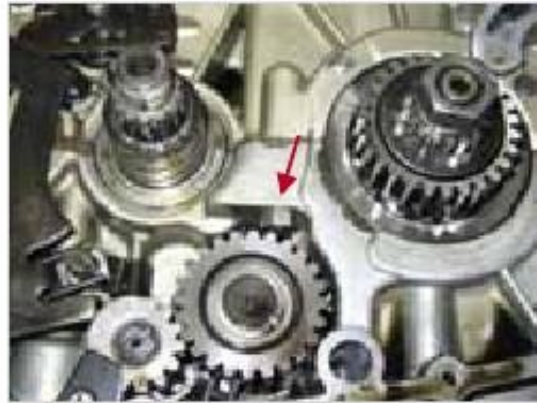
Figure 5-58: Loosen the screw behind the clutch basket
