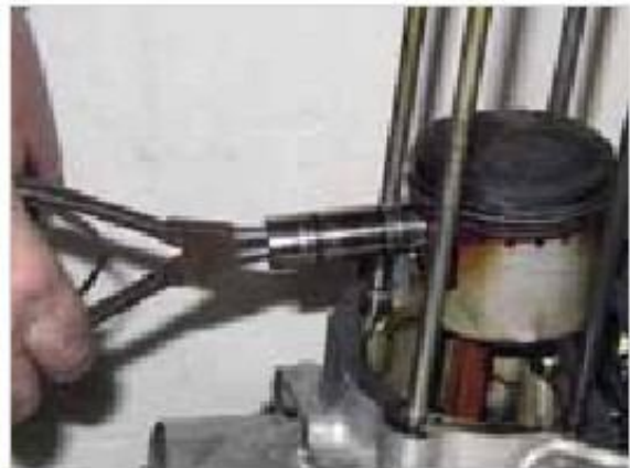
Figure 5-31: Pull out the piston pin
