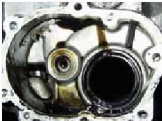
Figure 5-60: Remove the starter gear
