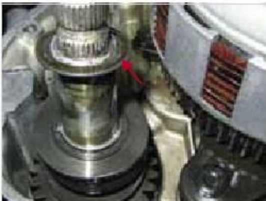
Figure 5-42: Pay attention to thrust washer, the kick starter shaft
