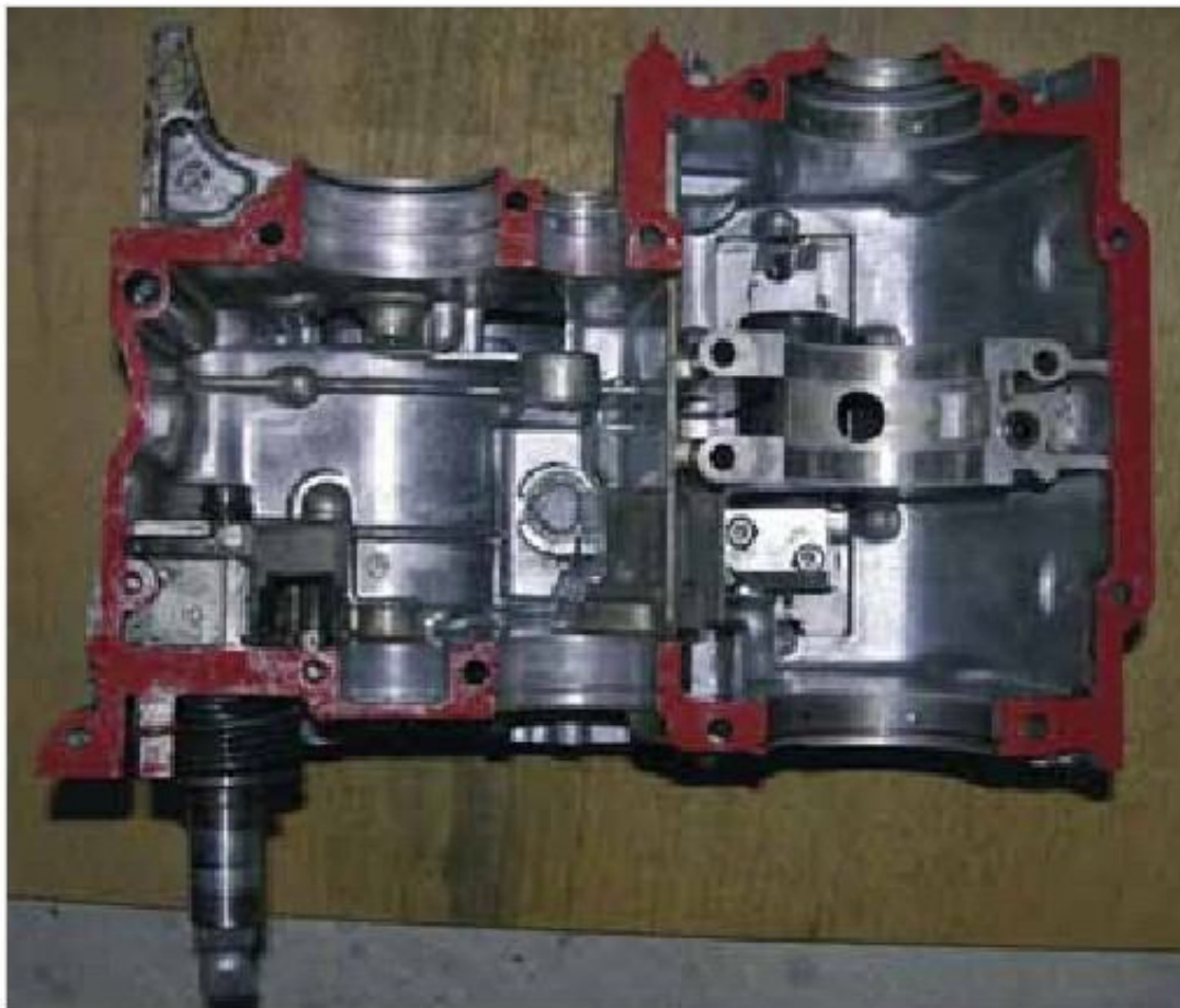
Figure 6-22: Lower half of the housing with sealant
