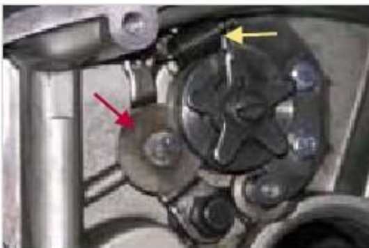
Figure 6-12: Gangarretierrad and spring mount
