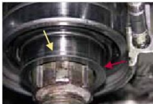
Figure 6-18: Bearing of the gearbox output shaft
