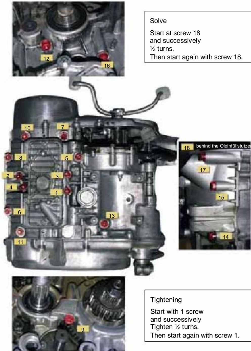
Figure 5-63: Tightening of the body screws
