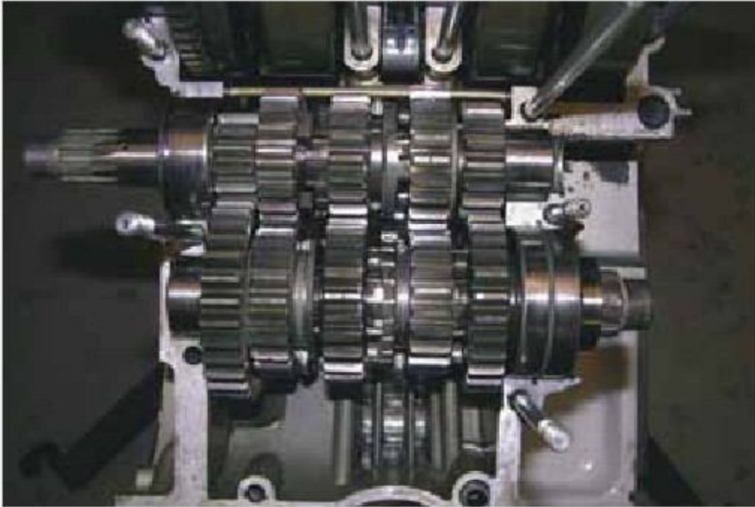
Figure 6-14: Insert the gear shafts
