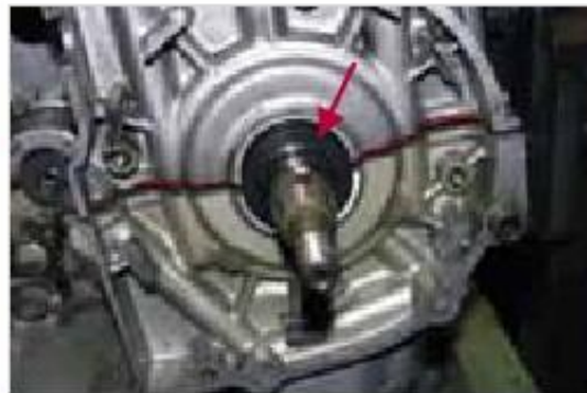
Figure 6-27: Transmission shafts with shaft sealing rings Figure 6-28: Crankshaft bearings with shaft sealing ring on the generator side
