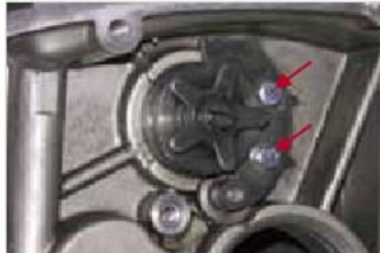
Figure 6-11: Retaining bar mounted
