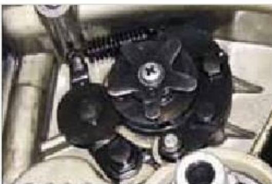
Figure 5-69: Unhook spring and Remove safety plate
