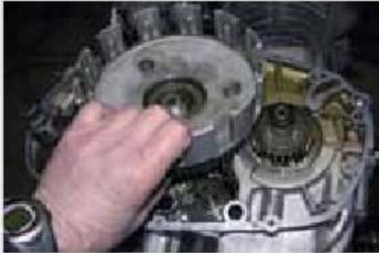
Figure 6-48: Clutch basket on Put gearbox input shaft
