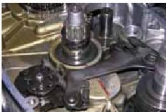
Figure 6-46: Put sleeve on transmission input shaft
