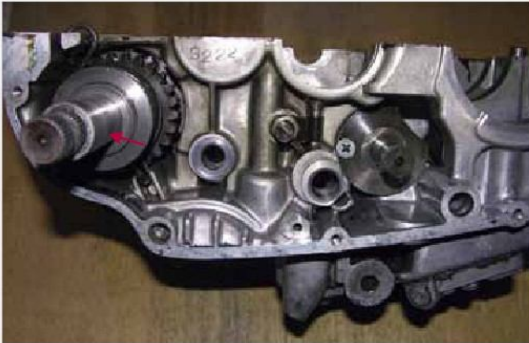
Figure 6-21: Kick starter mechanism used in the lower half of the housing
