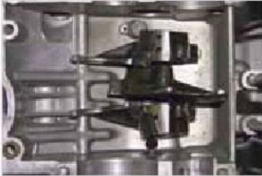
Figure 6-6: Insert the shift forks
