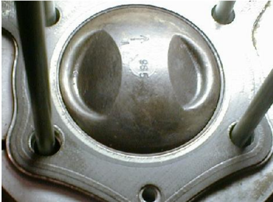
Stock (standard) piston at TDC (top dead center)
