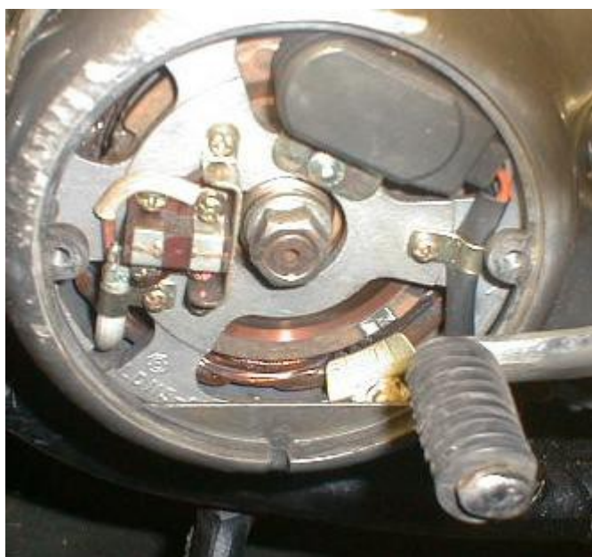
Rotor TDC mark on TDC "T" on RH side of timing tab plate 1980 and Up.
