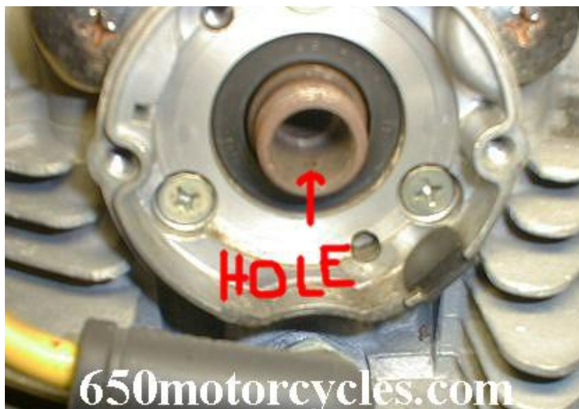
1980 Electronic Ignition Cam Still Has Points Index Pin Hole Above
