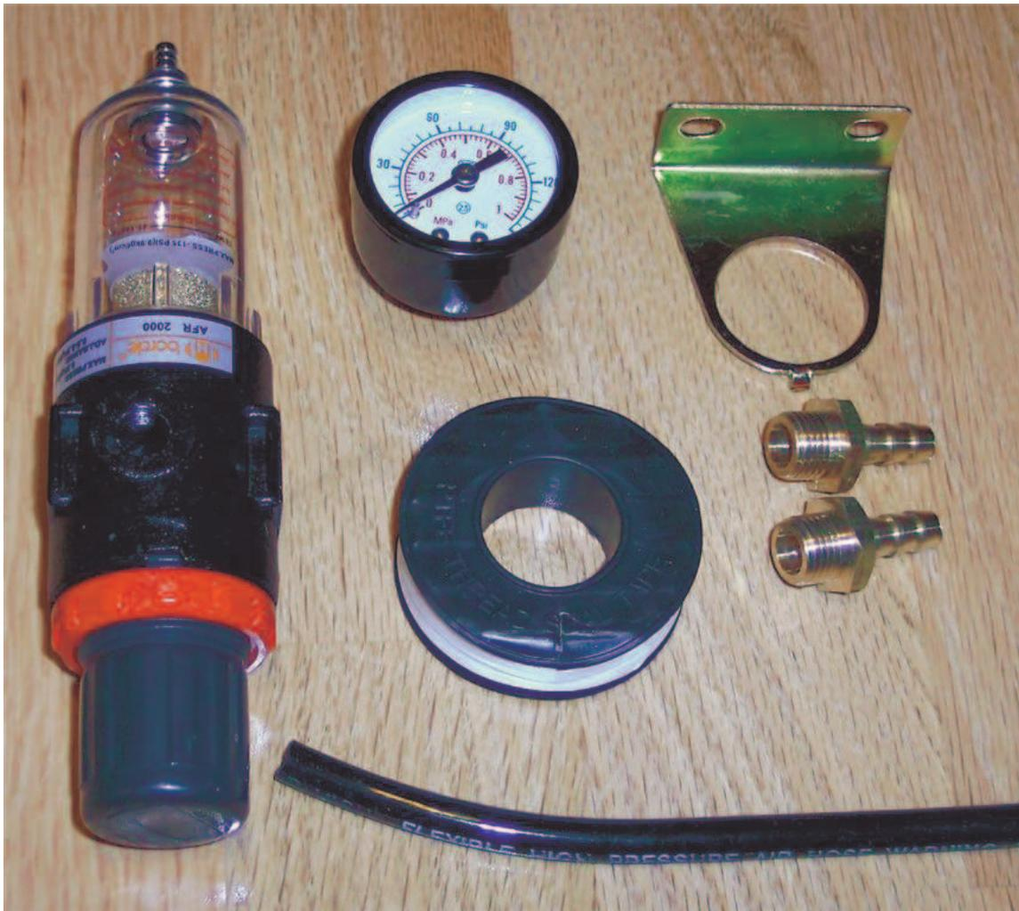
The gas, either air or argon, goes into one common pressure regulator/“moisture trap“, like the one above (which is woefully inadequate), before entering the machine. In its simplest form (like I built) you install pneumatic type quick connects to literally unplug either the air hose or argon hose upstream of the regulator to convert from TIG welding to plasma cutting.
