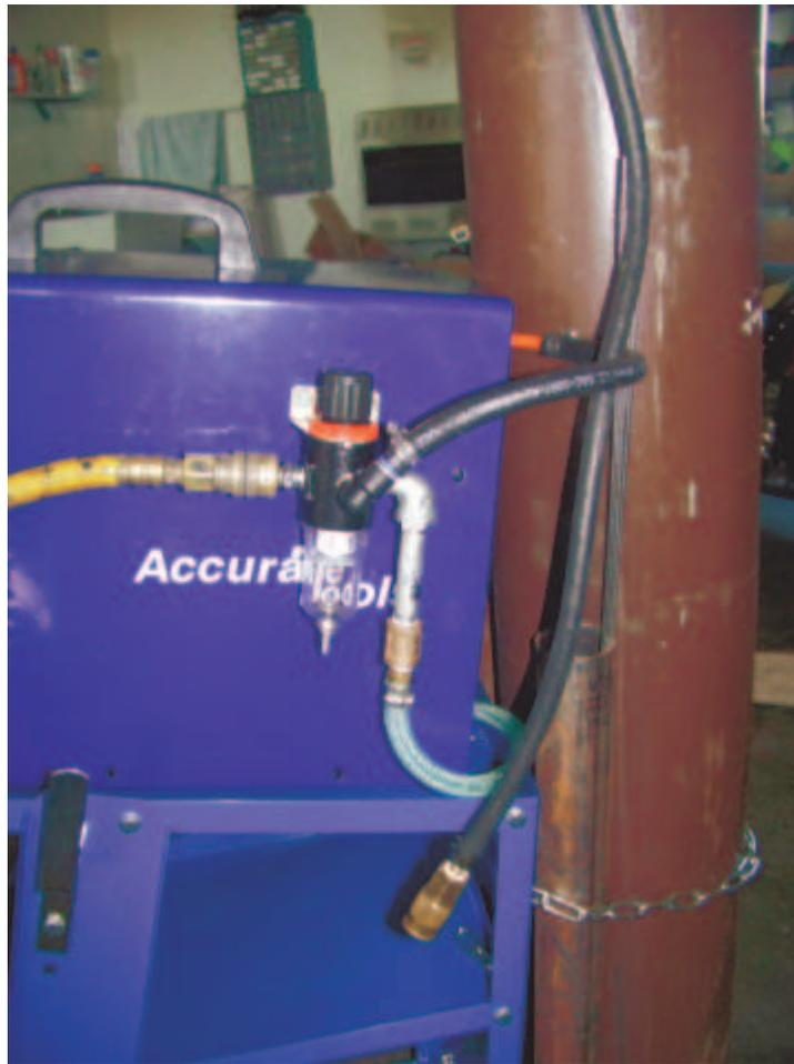
I drilled two holes in the welder cover (remove it, make sure you aren't going to short against anything!) and popped in two nut rivets. Those are like pop rivets except they are threaded 'nuts' instead of rivets. Very cool tool.
