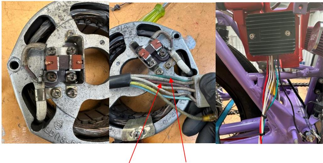
The red wire now grounds the inner brush to the stator and thus will be connected with the black ground from the Reg/rect unit. Green wire is from the outer brush; intend to connect to the Green wire from Reg/rect. Three whites are for the Reg/rect unit and the blue wire is not connected to the stator.
