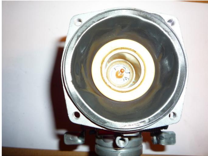
Finally you can fit the spring and the lid of the carburettor.
