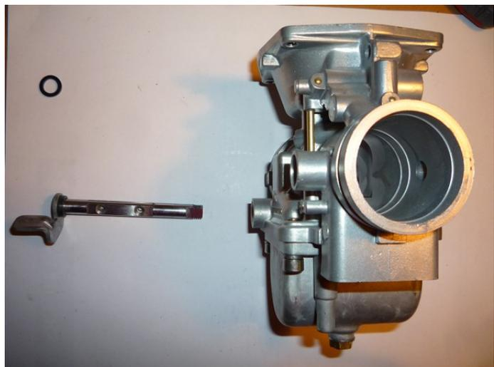
The actuating arm is also different compared to the #1 carb because it has an extension which rests on the throttle stop. Here I have lined up the parts in the order in which they are fitted to the shaft. Note that the plastic spacer goes on first, before the metal washer.
