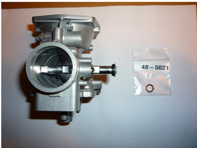
Next fit the throttle butterfly itself. This has to be oriented correctly because the edge of the flap is chamfered at an angle to match the throttle body. It's hard to see because of the camera flash, but there are some numbers stamped into the flap - these should face the front, underneath the shaft.
