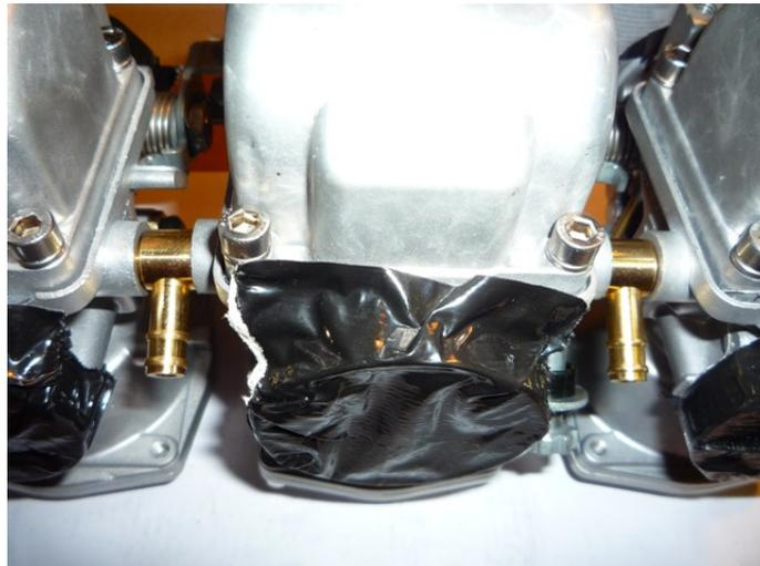
Next the mounting bracket, which holds the carbs firmly in place. I used Torx screws in place of the Philips screws that were there originally, mainly because I happened to have some lying around and because they don't chew up as easily as the originals.
