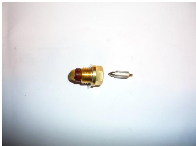
Fitting the float valve is a simple case of screwing it in and tightening (gently) with a 10mm spanner.
