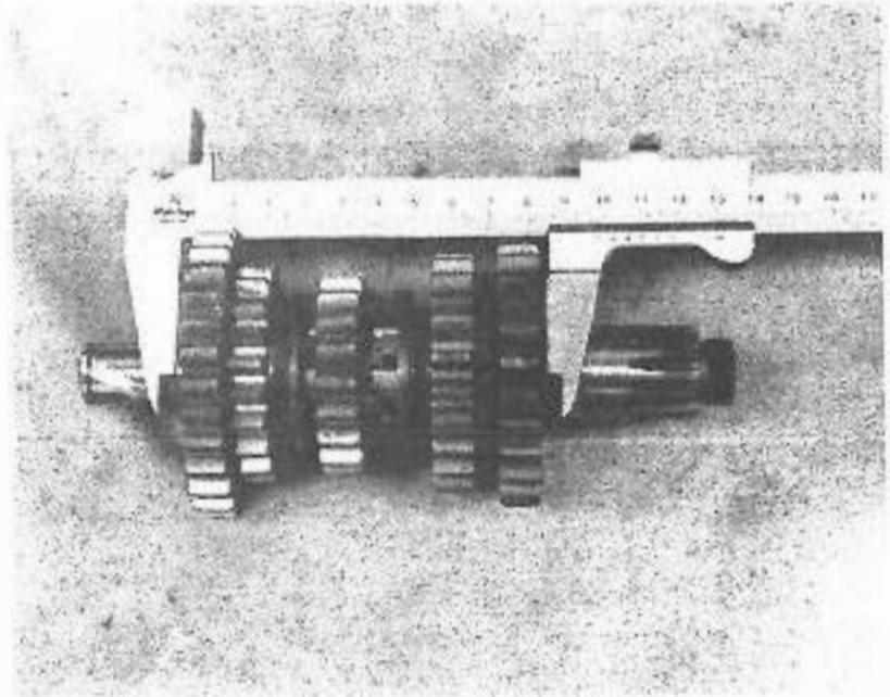
2. Measure transmission shaft length. Measure transmission axle length from one bearing contact surface to the other bearing contact surface (across gears and circlips, if any on the outer ends). Include standard shims usually included in the engine and listed in the parts book.
