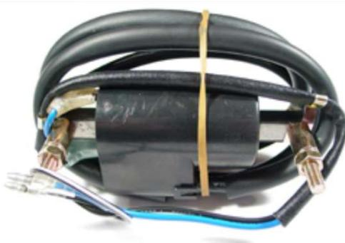
Dual Lead Ignition Coil for use with Single Contact Point Type Conversions or Early Type Boyer Digital Ignitions. 12 Volt, 4.5 Ohm Primary Resistance, 102mm c-c mounting points.
