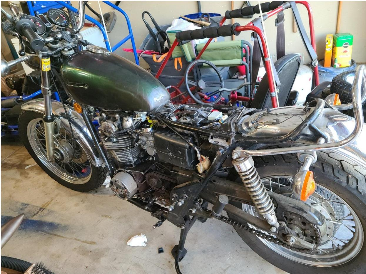
Given his declining health I decided to take over this bike from the beginning. So far, under his guidance, I have rebuilt the BS34s, performed general tuning on the engine (cam chain, valves, etc...), rewired several problem systems (rotor, turn signals, fuse box), rebuilt the frontend, brakes, clutch, filters,
