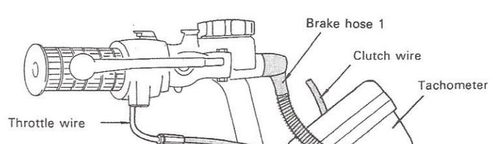
Pass throttle wire over tank fitting bracket, and pass clutch wire and wire harness R under the bracket.
