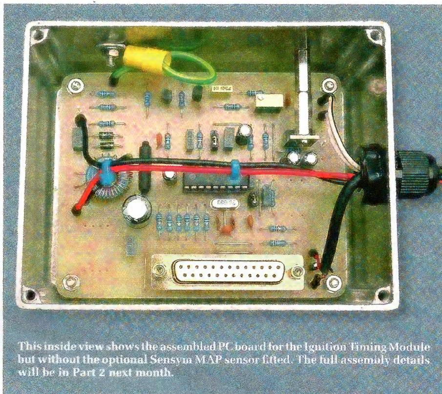
This inside view shows the assembled PCB for the Ignition Timing Module but without the optional Sensym MAP sensor fitted. The full assembly details will be in Part 2 next month.
