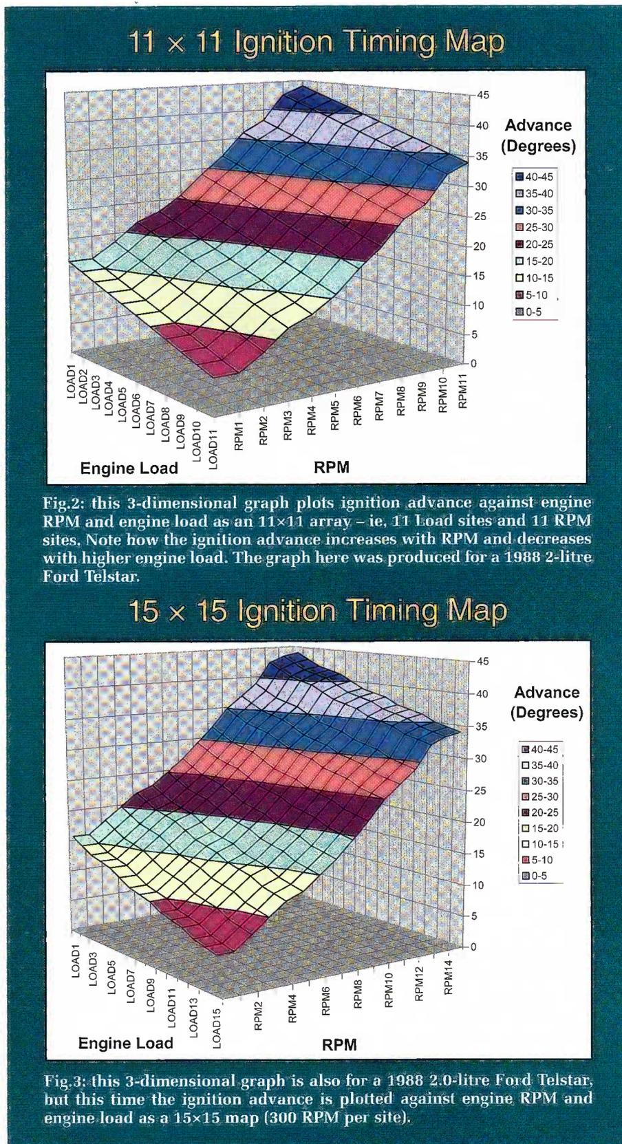
Fig.2: this 3-dimensional graph plots ignition advance against engine RPM and engine load as an 11×11 array – ie, 11 Load sites and 11 RPM sites. Note how the ignition advance increases with RPM and decreases with higher engine load. The graph here was produced for a 1988 2-litre Ford Telstar.
