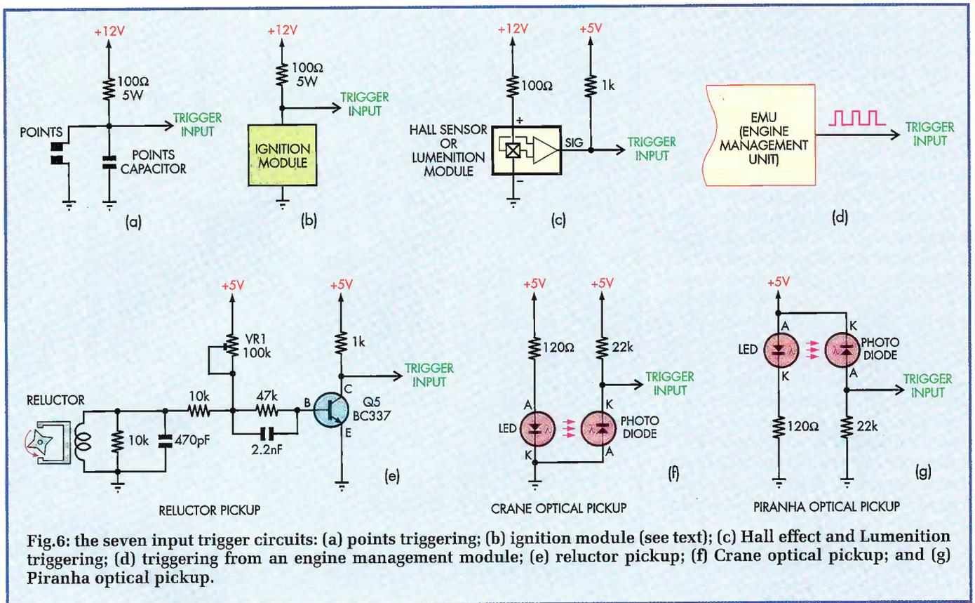
Fig.6: the seven input trigger circuits: (a) points triggering; (b) ignition module (see text); (c) Hall effect and Lumenition triggering; (d) triggering from an engine management module; (e) reductor pickup; (f) Crane optical pickup; and (g) Piranha optical pickup.
