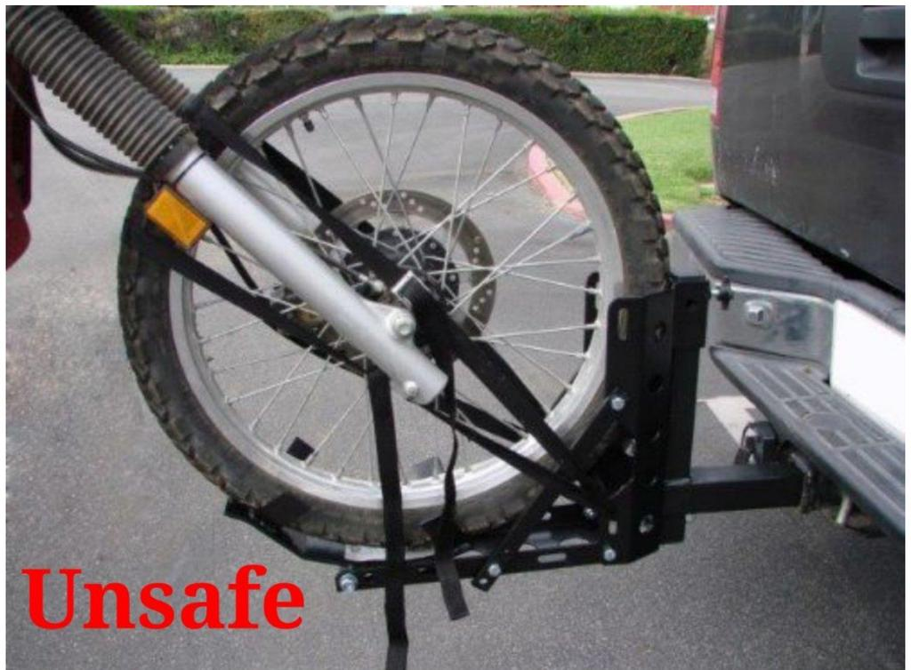
**The bike should be attached to the tow vehicle itself by the tie-down straps for safety.**
