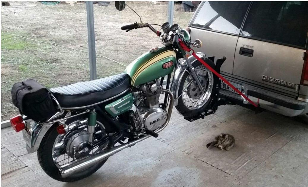
A proper tie-down is triangulated off to the sides, keeping the strap as parallel to the forks as possible. The tie-down strap is tightened while pulling one side of the handlebar down, compressing the forks a
