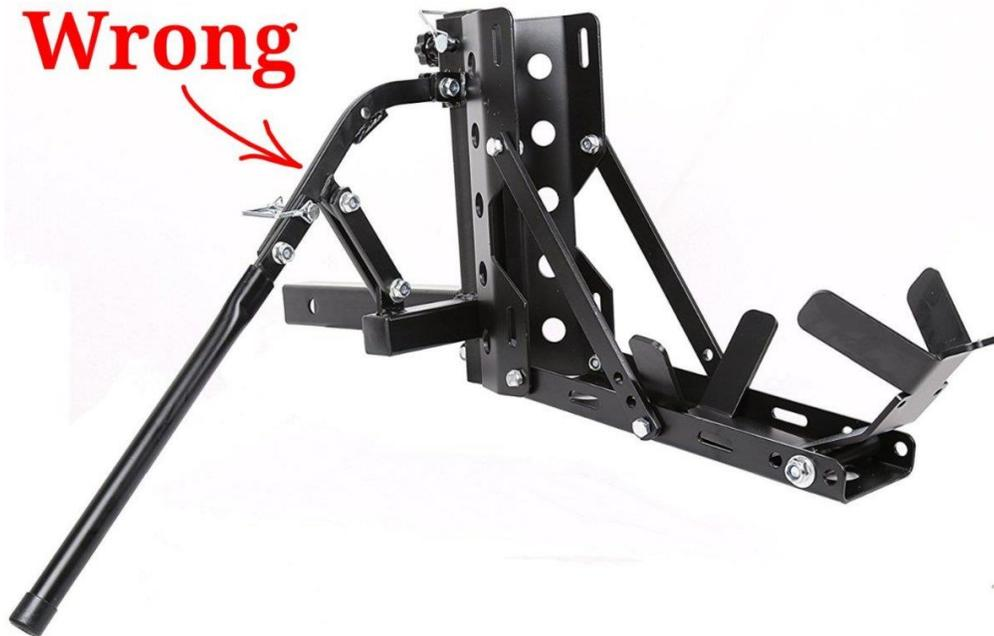
The unit won't work well, if at all, assembled that way. The proper lever arm assembly looks like this:
