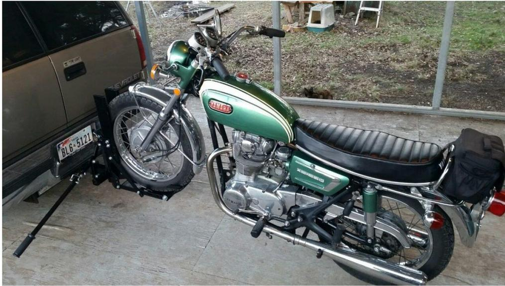
*Amazing* - the bike stays vertical and still resists any attempt to lean it over. The effort to lever it up to the travel position is quite reasonable. In fact, as the unit reaches the top of its travel, the lever ratio of the mechanism approaches infinity which means that the effort to "hold" it in the raised position is near zero (easily held with one hand) and so the other hand is free to insert the locking pin.
