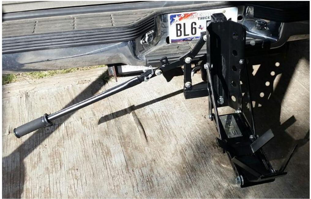
To put the handle into the “UP” position, just uncouple the handle's safety pin, swing it up to the travel position and reinsert the safety pin into the hole in the little tab.
