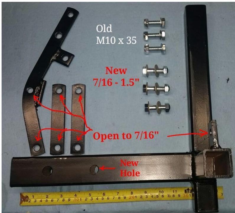
The pivoting front tire entry ramp is a sloppy fit. I figured that this could allow the front wheel to shift during the first part of bike loading and lifting, before the diagonal tie-downs are attached.
