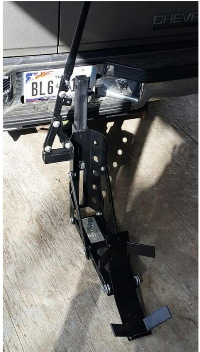
To raise the unit, just lever the handle down and the slider tray comes up – then insert the top safety pin.
