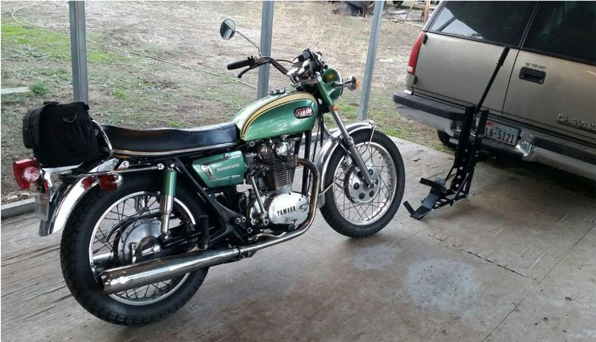
You just roll the bike onto and over the rocking entry ramp and the front tire just slides into the front channel and is sandwiched between those (2) 3/4" oak planks.
