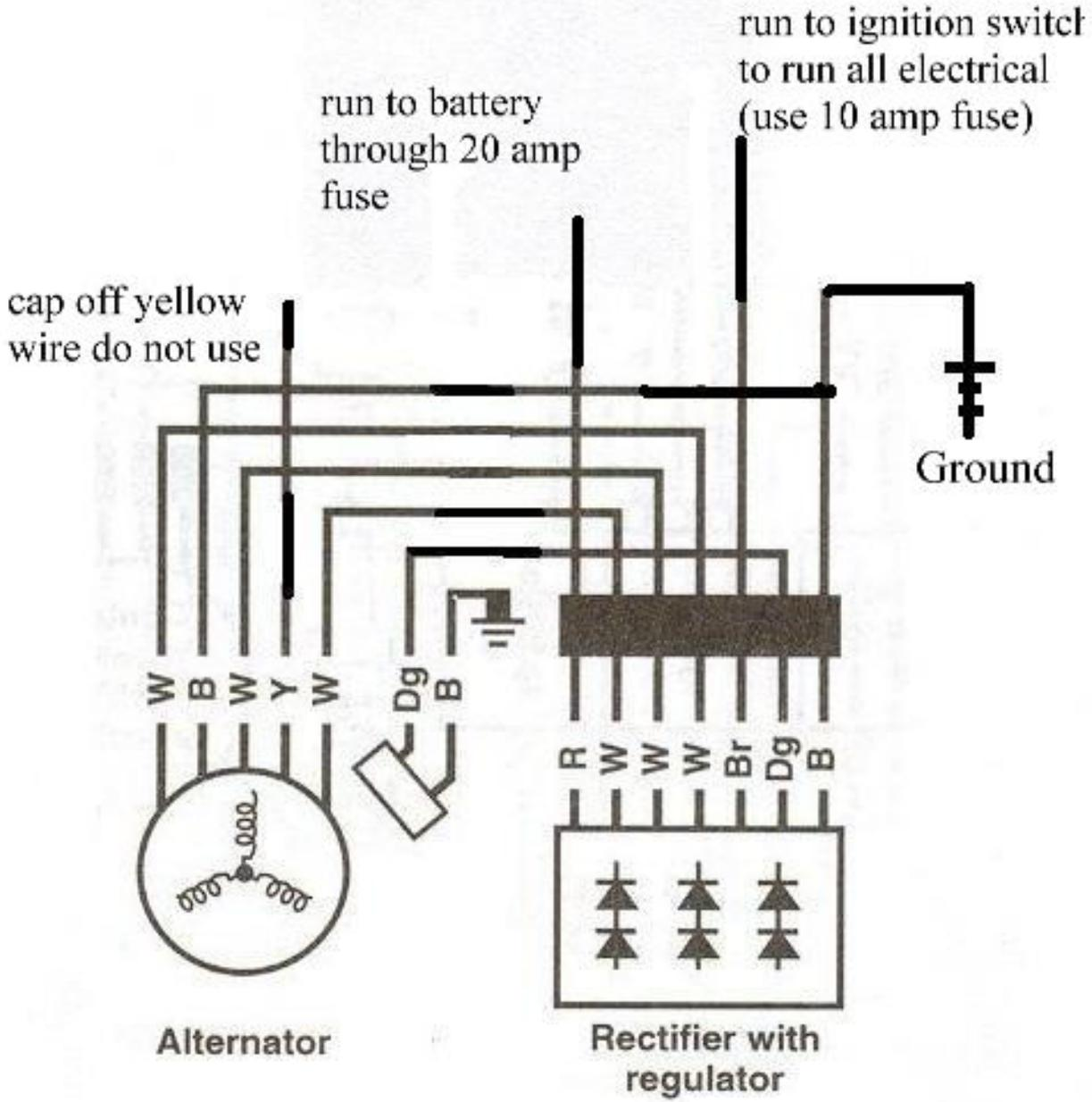
XS650 Charging System With Combined Regulator/Rectifier Simplified For Choppers
