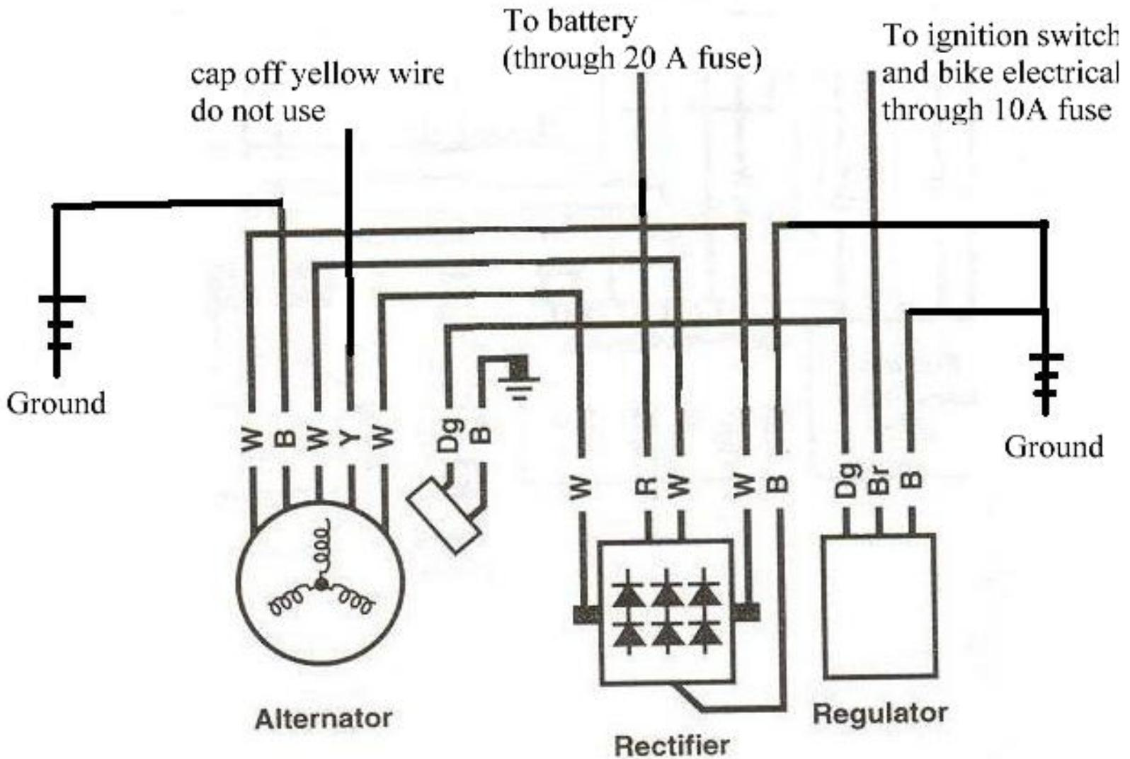
Older XS650 with separate regulator and rectifier
